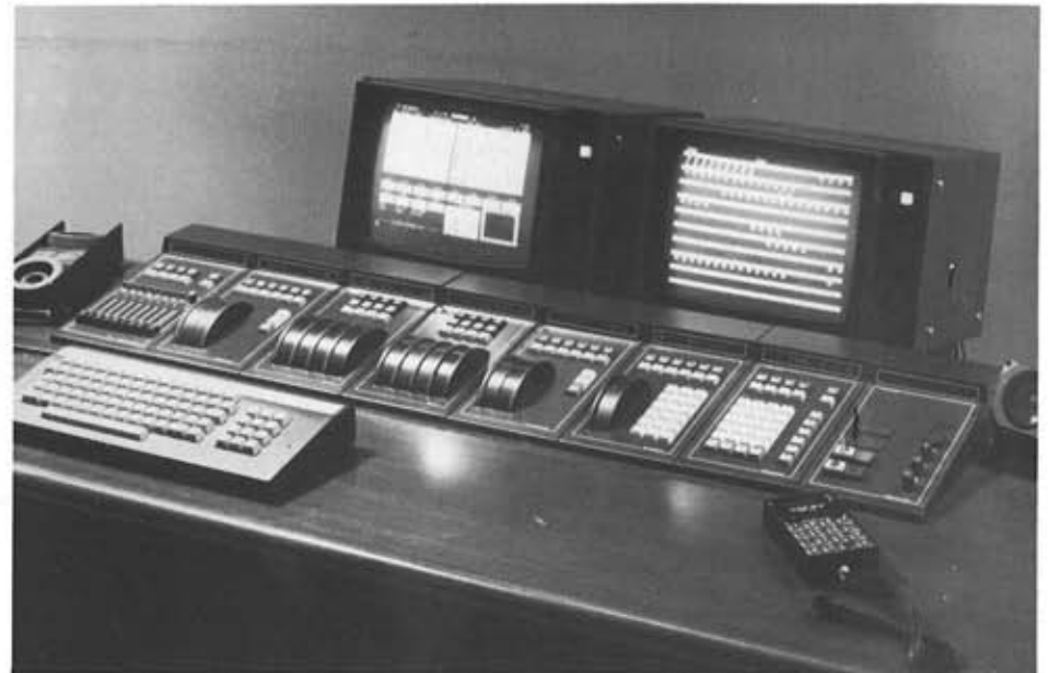
The Swedish-manufactured AVAB memory lighting control as recently installed in the Helsinki City Theatre, and used on the production of 'Cats'.
